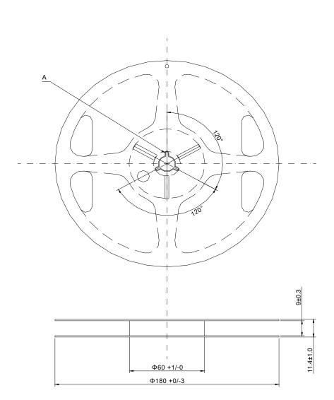
Material:Polystyrene (Conductivity) unit:mm
